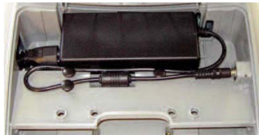
Mounting of the AC power adapter
